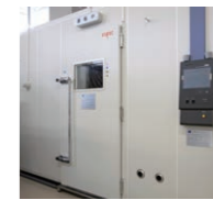
Environmental Test Room
