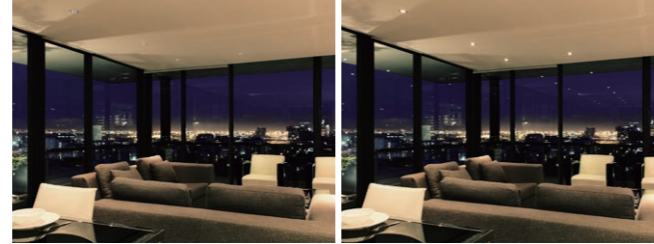
Glare-less mirrored cone Nighttime scenery looks even more appealing thanks to the reduction of glare on the window glass. General-purpose mirrored cone (silver) Glare readily appears on the window glass.
